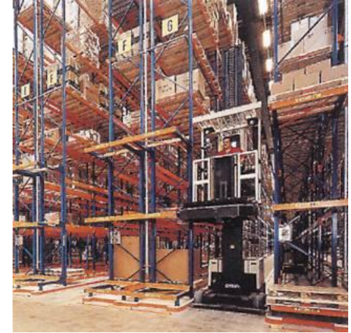
Alt 2: Narrow aisles; pallets 800 mm in depth
