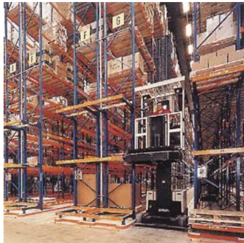
Alt 3: Narrow aisles; pallets 1200 mm in depth
