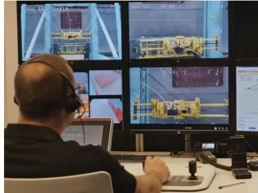
Figure 25: Remote container crane operations; instead of working alone on top of a container crane, the crane operators working on the Maasvlakte 2 terminals are working in an operating room. Source: YouTube: It's all about remote operations
