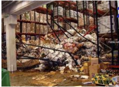
Forklift Collision with Storage Racks
