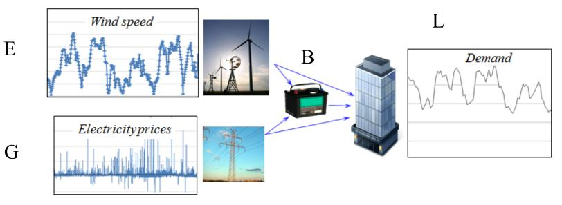
$$\begin{split} E_{t+1} &= E_t + \hat{E}_{t+1} \\ p_{t+1} &= \theta_0 p_t + \theta_1 p_{t-1} + \theta_2 p_{t-2} + \mathcal{E}_{t+1}^p \\ D_{t+1} &= f_{t,t+1}^D + \mathcal{E}_{t+1}^D \\ R_{t+1}^{battery} &= R_t^{battery} + x_t \end{split}$$
