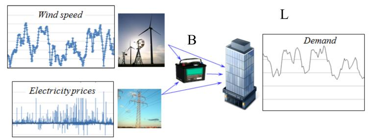
$$\begin{split} E_{t+1} &= E_t + \hat{E}_{t+1} \\ p_{t+1} &= \overline{\theta_{t0}} p_t + \overline{\theta_{t1}} p_{t-1} + \overline{\theta_{t2}} p_{t-2} - \overline{\theta_{t3}} x^{GB} + \varepsilon_{t+1}^p \\ D_{t+1} &= f_{t,t+1}^D + \varepsilon_{t+1}^p \\ R_{t+1}^{battery} &= R_t^{battery} + x_t \end{split}$$
