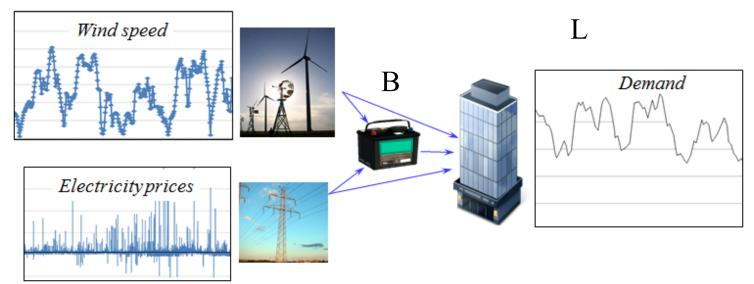
$$\begin{split} E_{t+1} &= E_t + \hat{E}_{t+1} \\ p_{t+1} &= \overline{\theta_{t0}} p_t + \overline{\theta_{t1}} p_{t-1} + \overline{\theta_{t2}} p_{t-2} + \mathcal{E}_{t+1}^p \\ D_{t+1} &= f_{t,t+1}^D + \mathcal{E}_{t+1}^D \\ R_{t+1}^{battery} &= R_t^{battery} + x_t \end{split}$$
